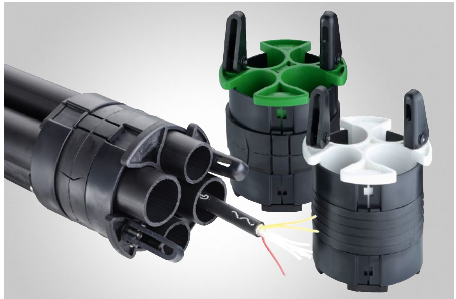
Divisible sealing and fixing discs AdSe-t seal the cavity between the cable duct pipe or half-pipe run and the multiple pipe.
